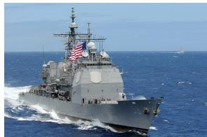
The *Ticonderoga* is a class of cruiser - the largest conventional (non-carrier) warship currently in the fleet. It was designed at the same time as the *Arleigh Burke* and it also is due for replacement. There are currently 6 active cruisers in the fleet and 10 in reserve out of a total class build of 27. However, four are to be retired this year. The Navy's plan is that a variant of the DDG(X) can serve as a Ticonderoga replacement.
